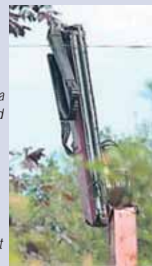
Overhead wires are a real hazard for loader cranes. A properly trained operator should be looking out for them.
