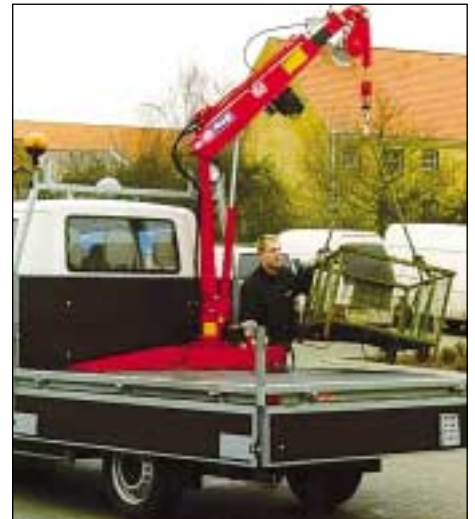
The smallest, compact lorry loaders are commonly fitted to builders' pick-up trucks and vans; sometimes have a lifting capacity of less than 500 kilograms.
